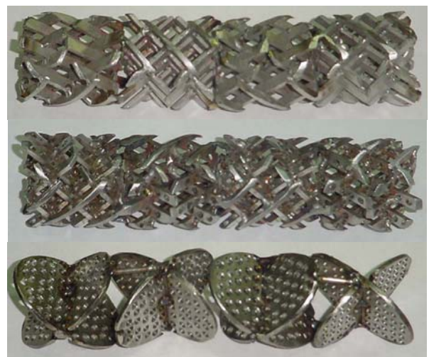
Fig. 1 Mixing elements of Sulzer SMX, YNU and YHC type with 4 unit elements
