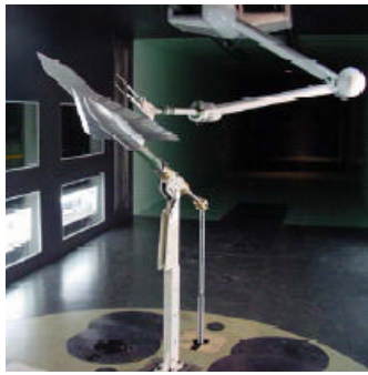
Fig. 3 Delta wing model in the test section of KAFA subsonic wind tunnel
