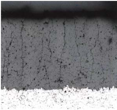
Fig. 9 Cross-sectional micrograph of the DVC-TBC coated layer (—— 0.3mm)
