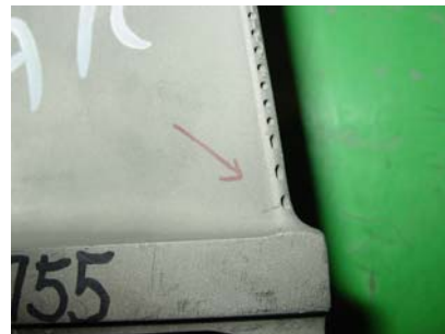
Fig. 5 No.1 Cooling hole crack
