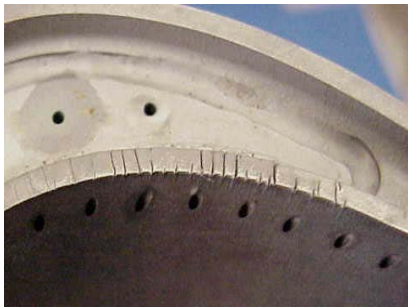
Fig. 3 Tip radial cracks occurred on the pressure side of bucket
