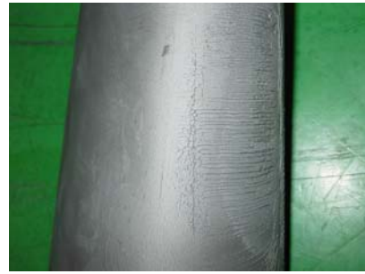
Fig. 4 Crazy cracks concentrated on the suction side airfoil and middle span of the bucket
