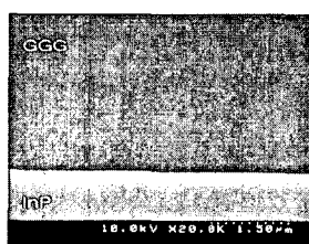
Fig. 2. SEM image of bonded sample between InP and GGG
