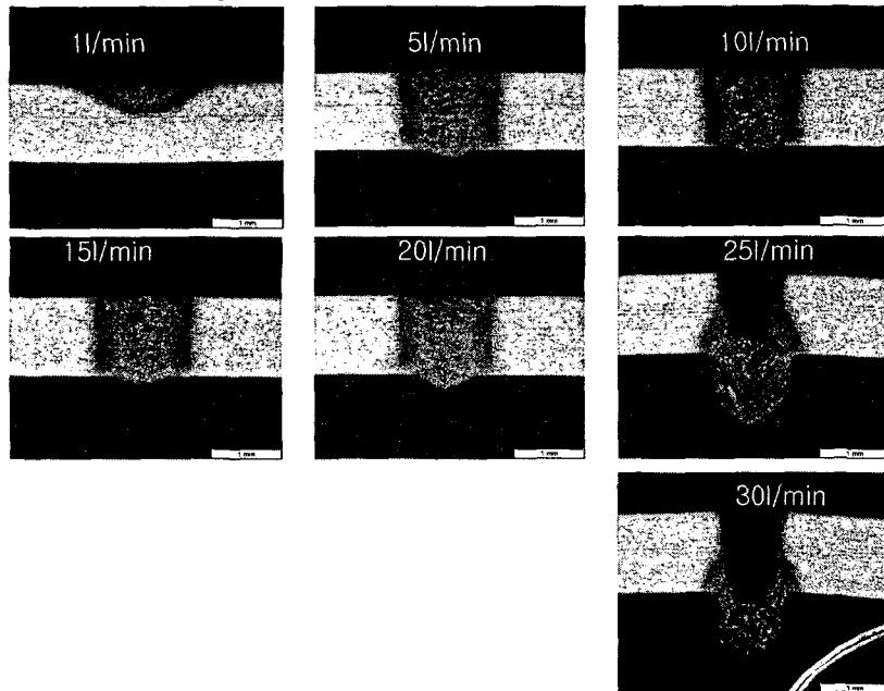
□ The effect of flow rate of Ar shielding gas on laser weldability of DP50 steels
