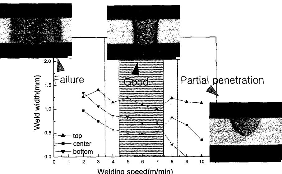
□ The effect of welding speed on Laser weldability of high strength steels(DP, TRIP, 45R, 60C)
