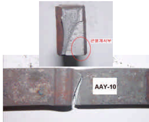
Fig. 9 Fracture surface of a welded specimen
