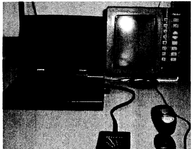
Fig. 2 Radar image capture system using PC camera
