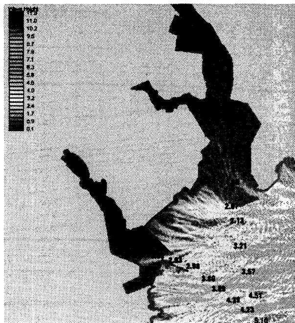
Fig. 9 Wave height predictions for the present configuration with wave conditions of 4.8 m and 8 sec, and wave direction of E (Nonlinear dispersion and wave breaking condition)
