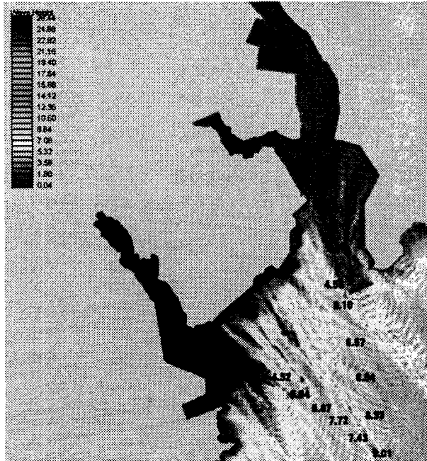
Fig. 7 Wave height predictions for the present configuration with wave conditions of 6.4 m and 10 sec, and wave direction of S (Nonlinear dispersion and wave breaking condition)
