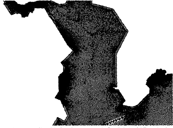
Fig. 5 Details of finite element mesh for Original Ulsan harbor
