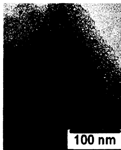
Fig.4 TEM photograph of CMS membrane dispersed with Pd nano particles with average diameter of c.a.5 nm.
