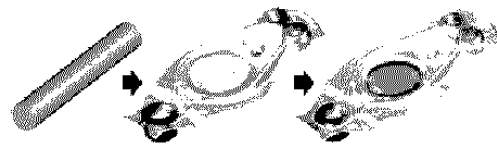
(a) Billet (b) Blocker process (c) Finisher process Fig. 2 Two forging processes for hot forging of the brake spider
