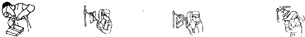
a) Flat Position b) Vertical Position c) Horizontal Position d) Over Head Position
