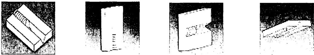
a) Flat Position b) Vertical Position c) Horizontal Position d) Over Head Position
