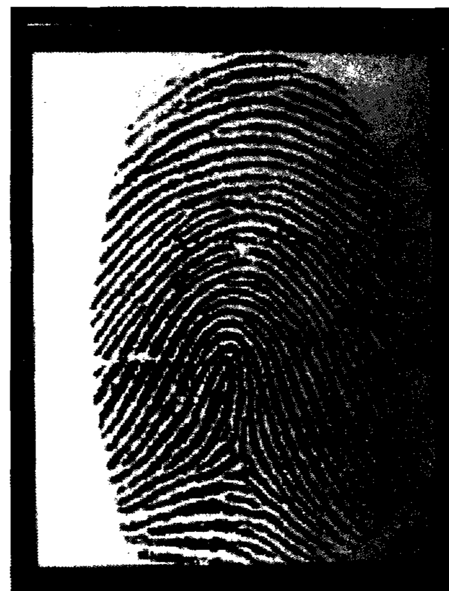
Fig. 4 A fingerprint image taken by our TFT FPS
