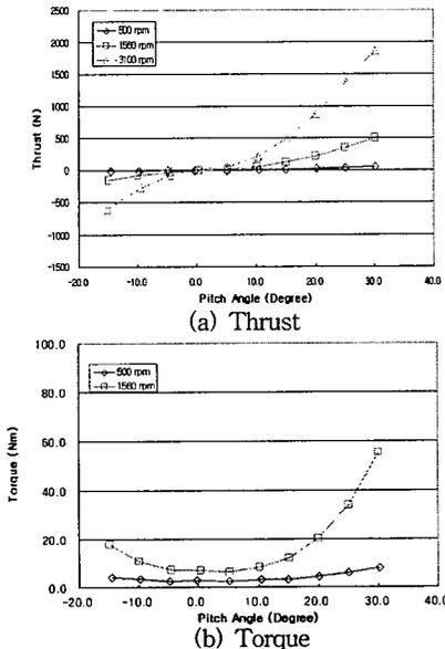
Fig. 10. Performance Test Results on Ground
