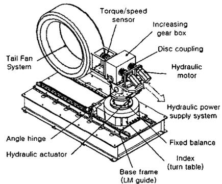
Fig. 3. ATS Test rig Design
