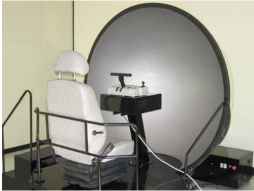
Fig. 4 Dome screen of the tilting simulator.
