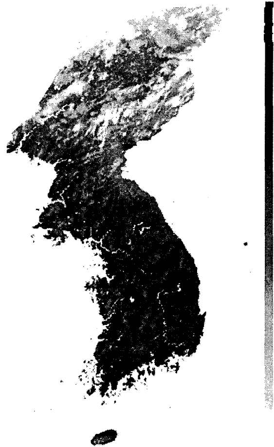
Figure 3. Sample image of LST retrieved from MODIS data using Price method for 12 August, 2004. Black indicates a warmer LST.
