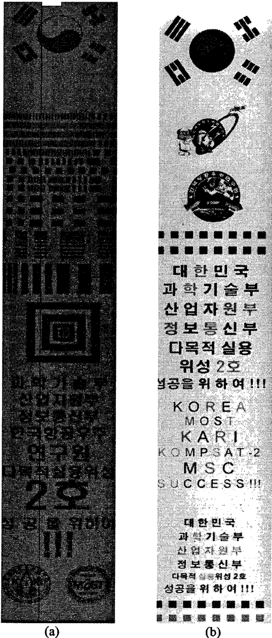
Figure 5 Output image. (a) PAN image of black and white input target (b) MS image of color input target.
