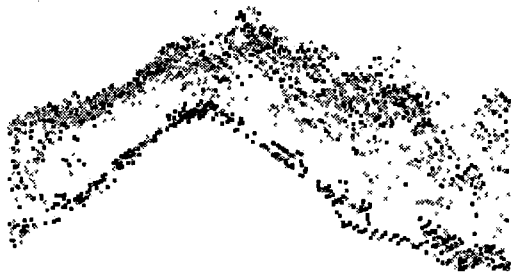
Figure 2. Vertical profile of the lidar pulse hit of the last returns (black) as compared to the first return (grey tone).
