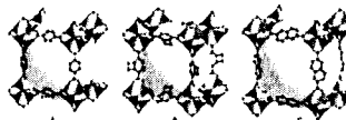
Single-crystal X-ray structures of MOF-5(A), IRMOF-6B, and IRMOF-4(C). Zn (blue) and O (red) spheres; C (black) spheres
