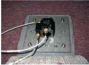
Fig. 4 vibration accelerometer
