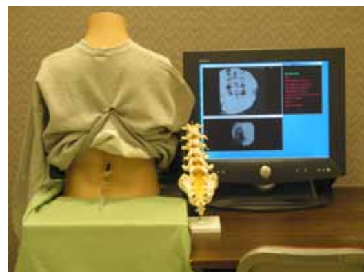
Figure 4. VR based Epidural anesthesia trainer. The robotic device is inside of human mannequin and it is connected with the syringes
