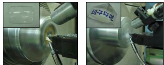
Fig.8 Machining of PMMA lens and prism by SPDTM
