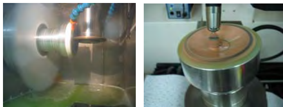
(a)Machining of BK7 by SPDTM (b) Polishing of aspheric lens by KRP-2200F
