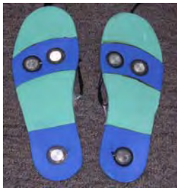
Fig. 2 Insoles in which shear sensors were inserted
