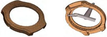
Fig. 4 Element model and delivery system for watch case simulation
