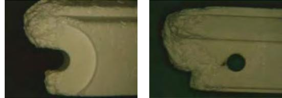
Fig. 6 The flow pattern around pin in experiment.
