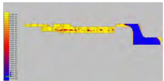
Fig. 6 Inside temperature of valve body on the solid time
