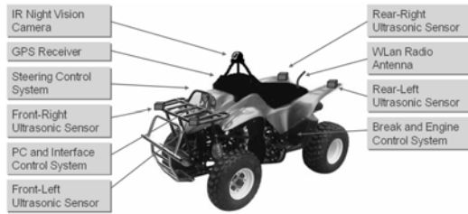
Fig.1 Field Robot System
