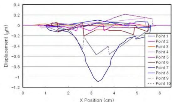
(b) Vertical Minimum Amplitude of Beam 1
