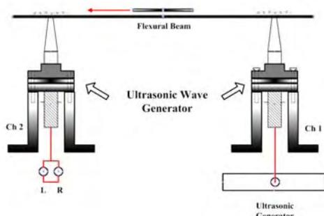
Fig. 1 Layout of Ultrasonic Object Levitation Transport System
