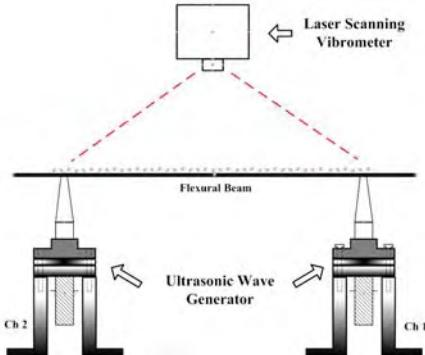
Fig. 2 Experimental Apparatus for Ultrasonic Object Levitation Transportation
