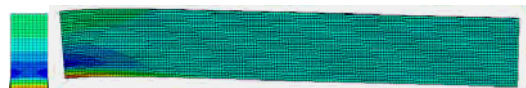
Fig. 10 Contour plot of residual stresses in bi-material metal joint with one material in elastic range and the other in plastic range (deformation scale factor: 190.804)
