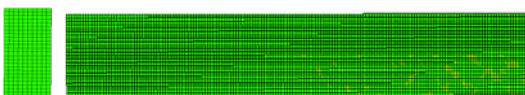
Fig. 7 Contour plot of residual stresses in elastic range of bi-material metal joint (deformation scale factor: 1)
