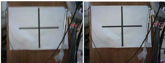
Fig. 4 Comparison of image on vibration before and after installing vibration absorber
