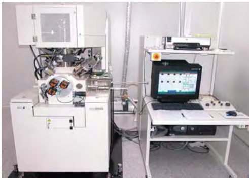
Fig. 1 FIB Photograph made by SII Nanotechnology Inc.(Model : SIM2050)
