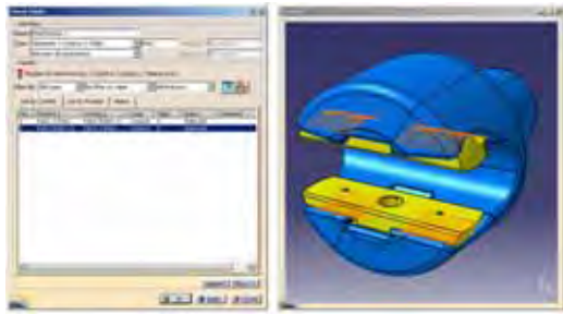
(b) Space analysis of top spindle and slipper metal
