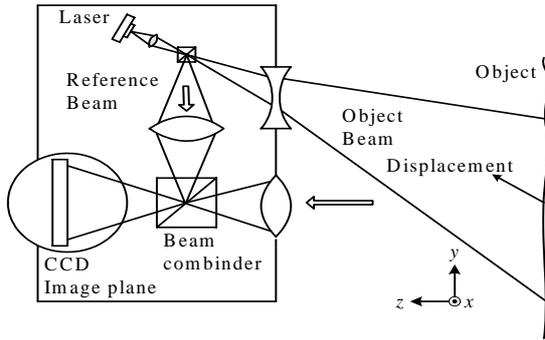
Fig. 1 Out-of-plane displacement sensitive ESPI interferometer
