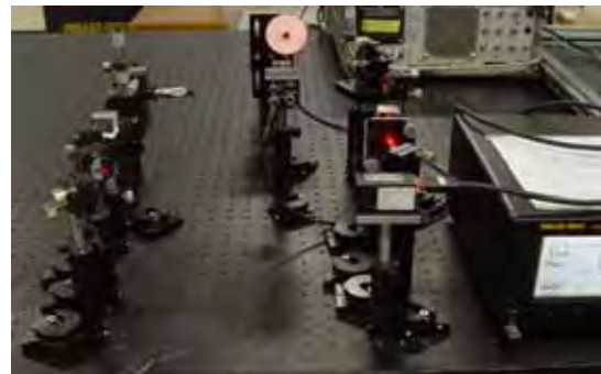
Fig. 3 Experimental setup of LD-SPM interferometer
