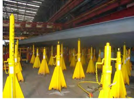
Fig. 2 Set up pin jig for ship block assembly
