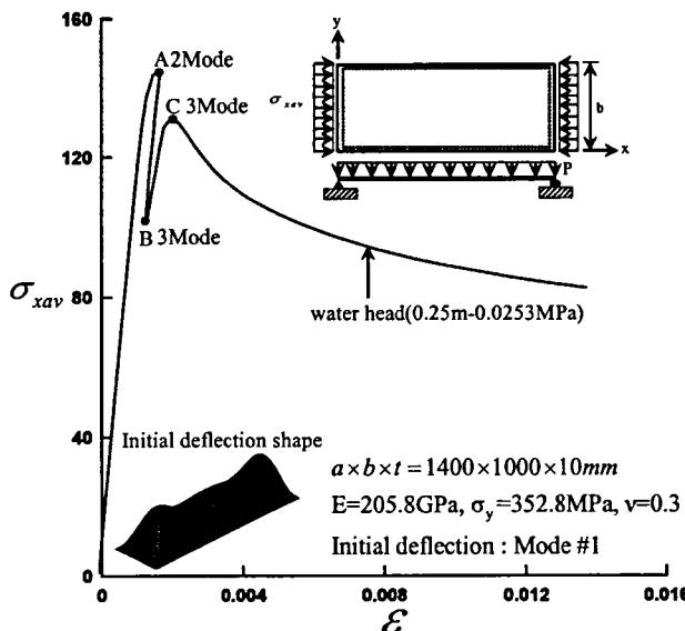
Fig.11 Secondary buckling behavior with thin-horse mode under lateral pressure load and uniaxial compression for aspect ratio 1.4
