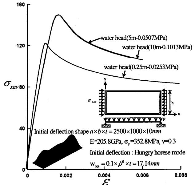
Fig.13 Comparison of compressive stress-strain curves with hungry-horse mode for aspect ratio 2.5
