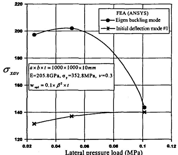
Fig.7 Comparison of compressive stress versus lateral pressure load according to the initial deflection type for aspect ratio 1.0
