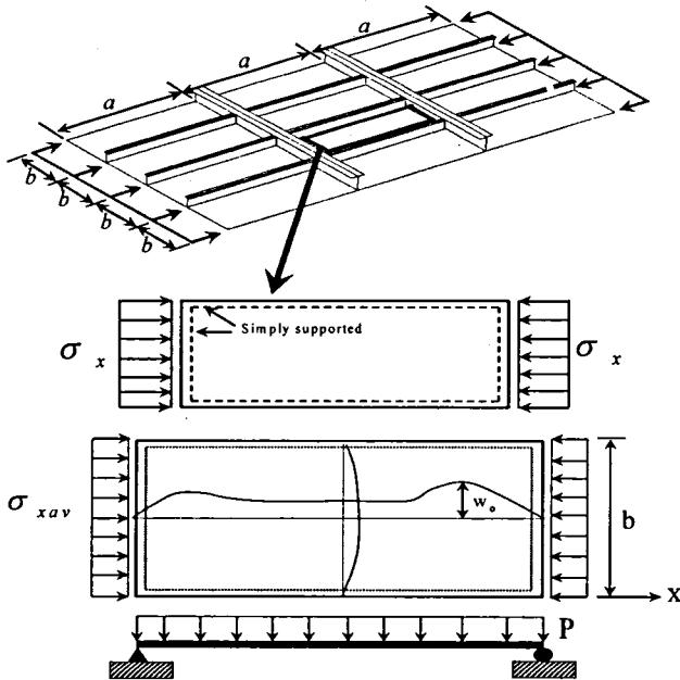
Fig.2 A simply supported plate with non-symmetric initial deflection under uniaxial compression and lateral pressure load
