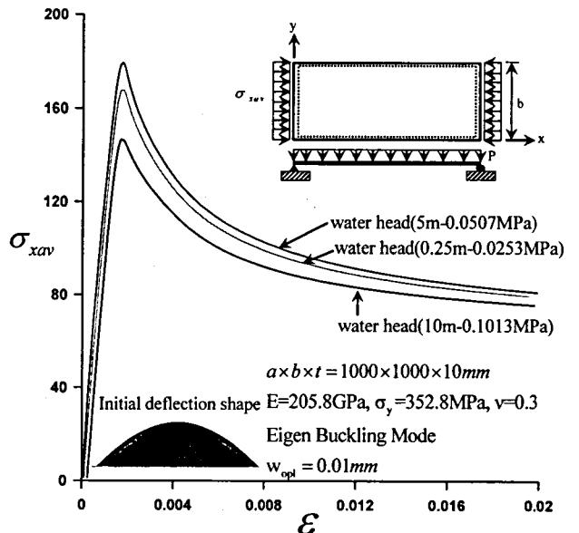
Fig.4 Comparison of compressive stress-strain curves with small initial deflection for aspect ratio 1.0
