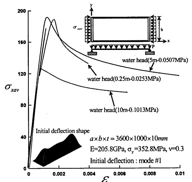
Fig.14 Comparison of compressive stress-strain curves with hungry-horse mode for aspect ratio 3.6
