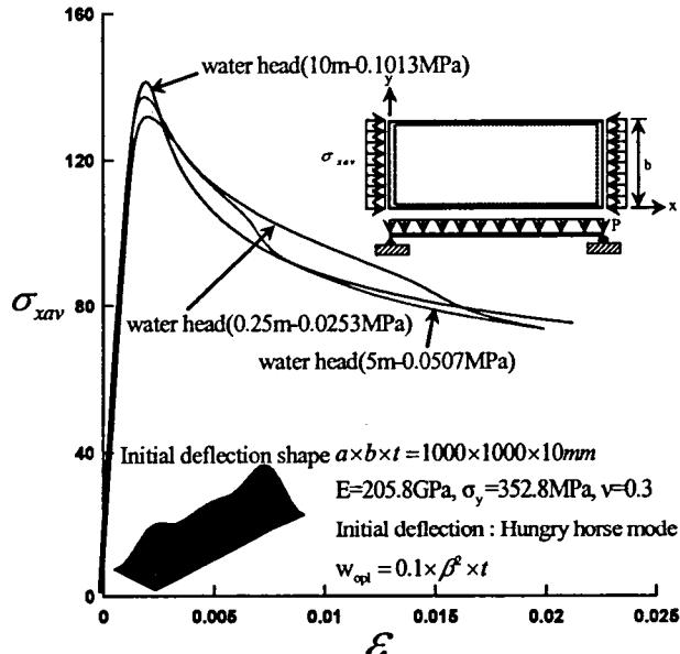
Fig.8 Comparison of compressive stress-strain curves with hungry-horse mode for aspect ratio 1.0
