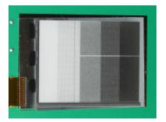
gray-scales are successfully shown. Although the reason that more than 6 image frames is needed is not yet clear, the flexible AM-EPD device still
