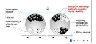
negative electric voltage is applied to a bottom electrode, the black particles are attracted to the top transparent electrode, where they become visible to the user as a black spot. White spots can be seen when the opposite polarity of voltage is applied.
