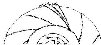
Fig. 5 Changing the outlet blade angle.
