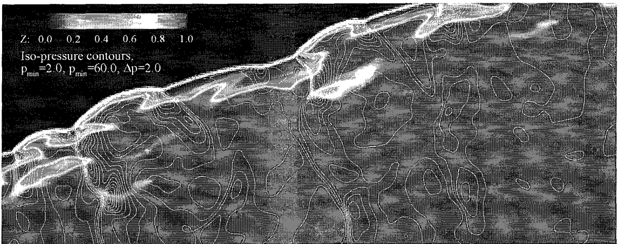
Fig. 5 Unstable oblique detonation wave surface. Locally magnified plot of a region in Fig. 4.
