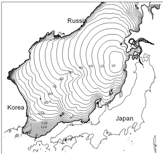
Figure 1. Contour of arrival time of leading tsunami (unit: minutes)
