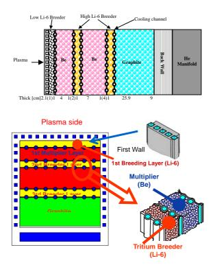
Figure 2. Conceptual design of HCSB
