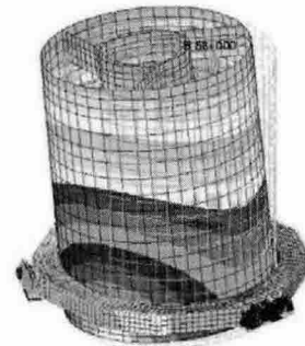
(Fig. 3.4 The 2nd bending mode of model (I), 45.1Hz)
