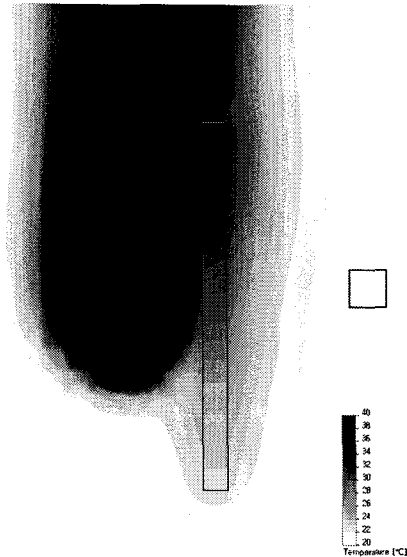
Fig. 3 Air temperature distribution for 500°C source without thermal radiation (case 5)
