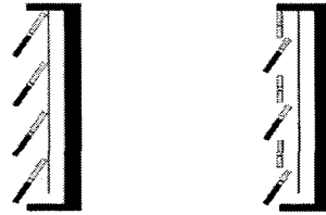
Fig. 2 The former and the alternative working modes during day in summer.
