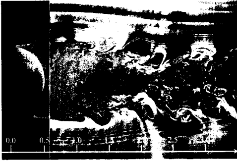
Fig. 3 Smoke-wire flow visualization of sphere wake
