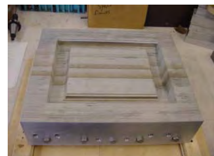
Fig. 8 PEL thermoforming mold with three conformal channels.
