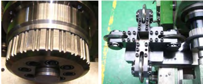
Fig. 4 Mandrel on spindle and rolls on turret used in the spinning experiments
