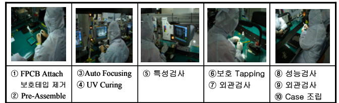
Fig. 2 Working processes of phone camera module
