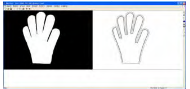
(e) Original image and sewing line after erosion of 8 times and edge extraction
