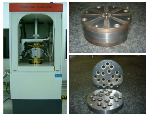
Fig. 3 Molding Press GMP207Hv and Mold
