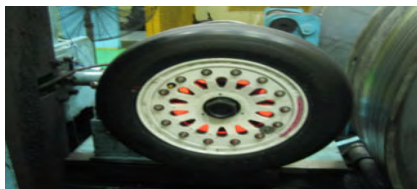
Fig.3 braking test at Inertia dynamometer
