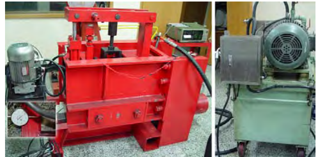
Fig. 1 Experimental apparatus to test a performance of the wedge type rail clamp
